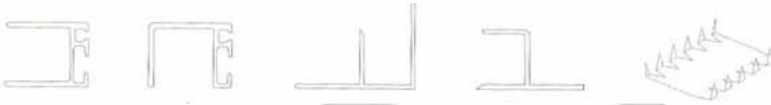
H-shape PVC flange; Vertical PVC Flange; F-shape alloy flange; Y-shape alloy flange; U-shape tiger
